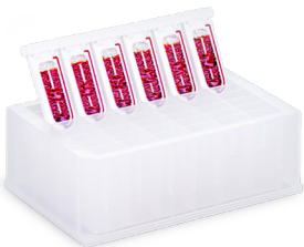
MD1000 cartridge in 48-deep well plate
