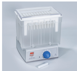
Figure 9 | XDB Dialysis Box with magnetic stirrer
